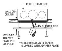
• Mounting to a 4S electrical box with 404 plaster ring
